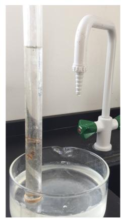
Oxygene reacts with iron – and makes it rust. As the Glastube with
